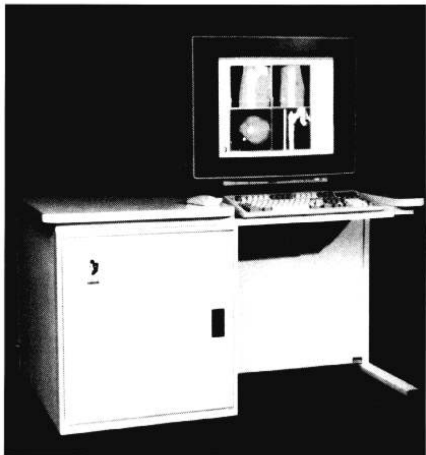
Figure 5. The ORTHODOC workstation has four quadrants that display images of the patient's femur, the prosthesis, and the bone motion rod.
