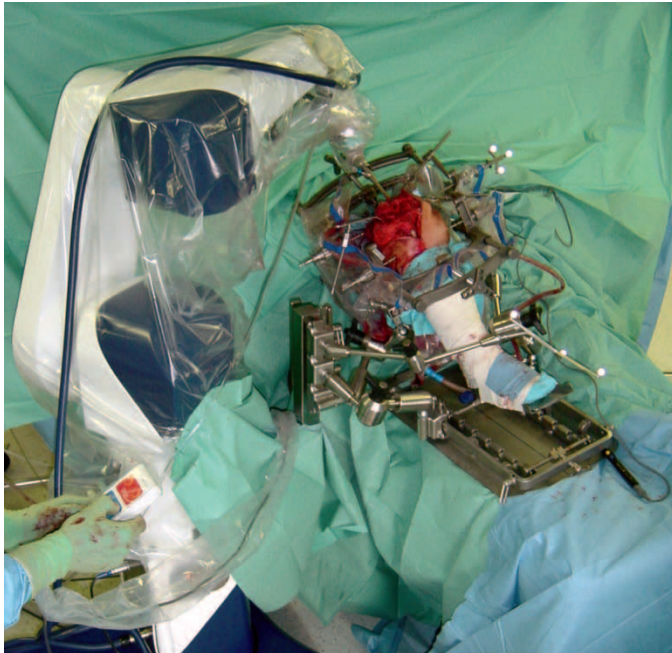
Figure 2. The robotic arm moves with six degrees of freedom. It is draped sterile and equipped with a high-speed milling tool. Threaded Steinmann pins are placed through the proximal tibia and the distal femur from medial to lateral. The pins are clamped taut in a metal frame. The frame and the sterile thigh holder are rigidly connected to the robot itself. Relative motion between the robot and the knee joint is thus minimized. Two sets of reflecting spheres are connected to the robot and the knee joint, and are constantly monitored by an infrared camera which is ready to stop the milling in case of excessive bone motion.
