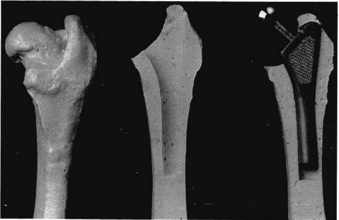
FIG. 1. The robotic system machines dimensionally accurate cavities. This photograph (left to right) shows an intact foam bone, a cut-away view of a robotically reamed foam bone, and a cut-away view of a foam bone with implant inserted.
