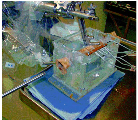
Figure 2. Water tank with cadaver bone mounted on the robot.
